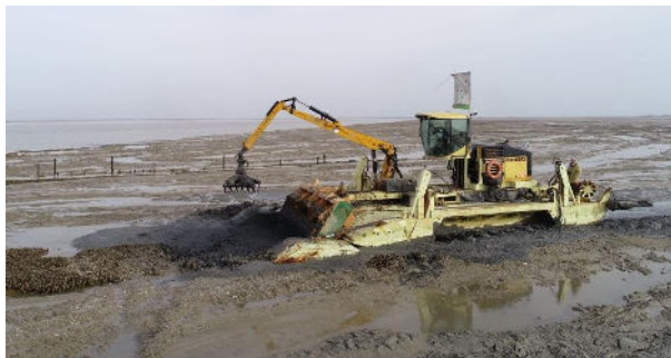
Figure n°8: Amphibious excavator in action to restore mudflats
